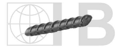
The American Welding Society (AWS D 1.4) sets out the practices for welding rebar in the U.S. Without special consideration, the only rebar that is ready to weld is W grade (Low-alloy — A706). Rebar that is not produced to the ASTM A706 specification is generally not suitable for welding without calculating the "carbon-equivalent."
